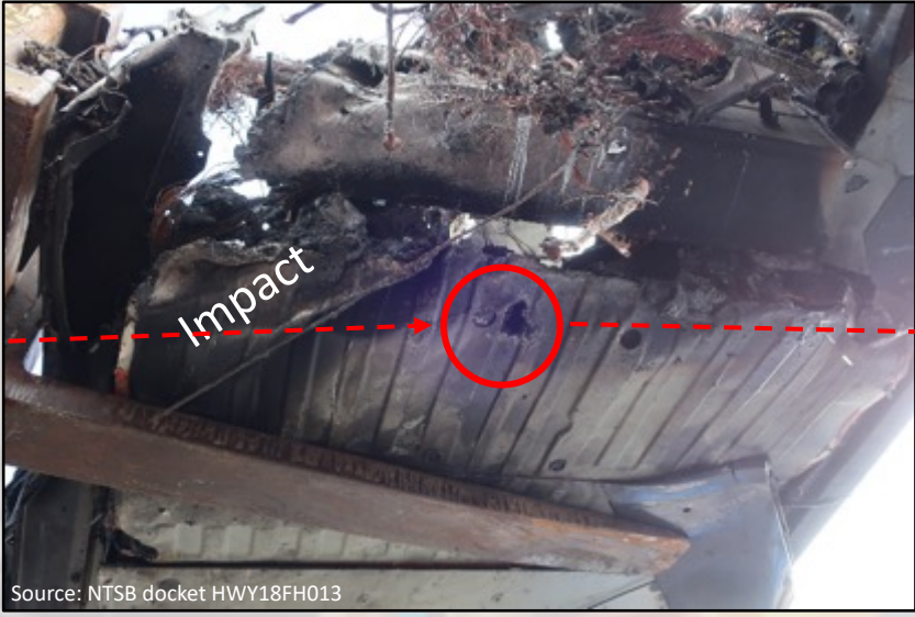
Arc flash hole into passenger footwell
