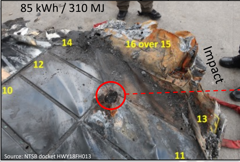
5" Arc hole found through top of battery
