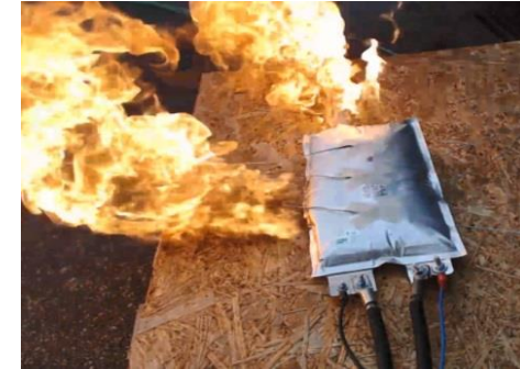
Overcharge abuse with a 2 C-rate current of a 30 Ah cell with LATP/NCA. ( \text{LiAlTiPO}_4 - \text{LiNiCoAlO}_2 )
