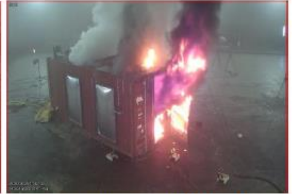
Flashover and flaming from open door [TR + 02:09:48]
