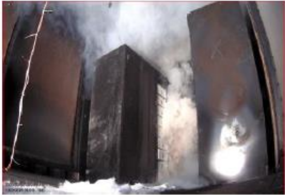
Smoke accumulation at second smoke detector activation [TR + 00:00:55]
