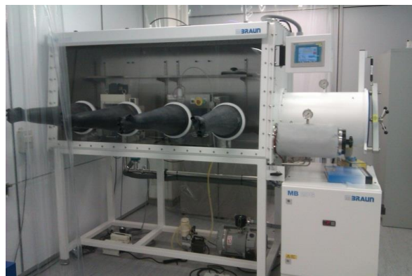
Glove box to fill electrolyte and crimping
