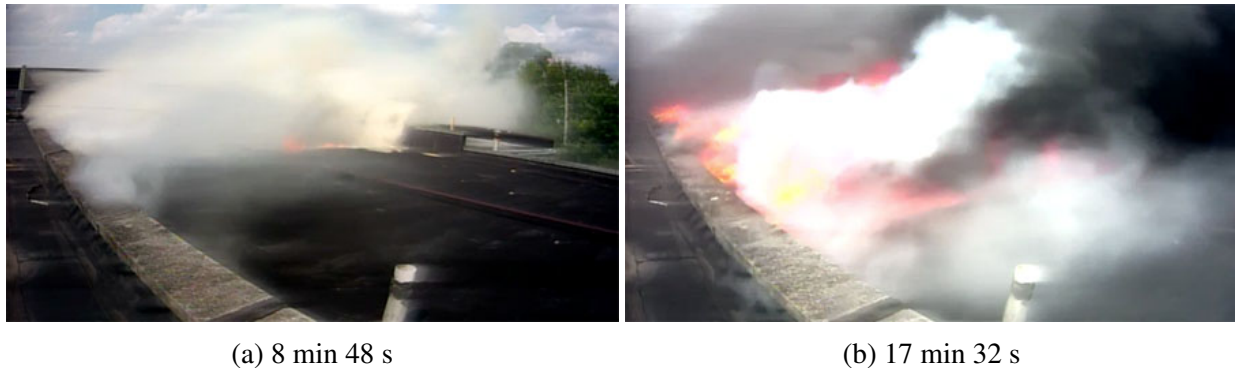
Figure 3.19: Images from the camera on the CD corner showing the ignition of the roofing material.
