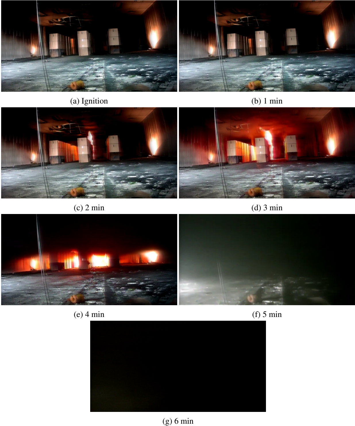
Figure 3.14: Sequential interior images during Experiment 2 looking toward side C from the side A. The interior camera was lost after 6 min due to thermal damage from the fire.
