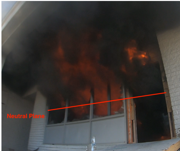
Figure 3.29: View of the front of the unit from the exterior camera 4 min 30 s after ignition, 30 s after ventilation occurred, during Experiment 3. The red line illustrates the approximate location of the neutral plane.
