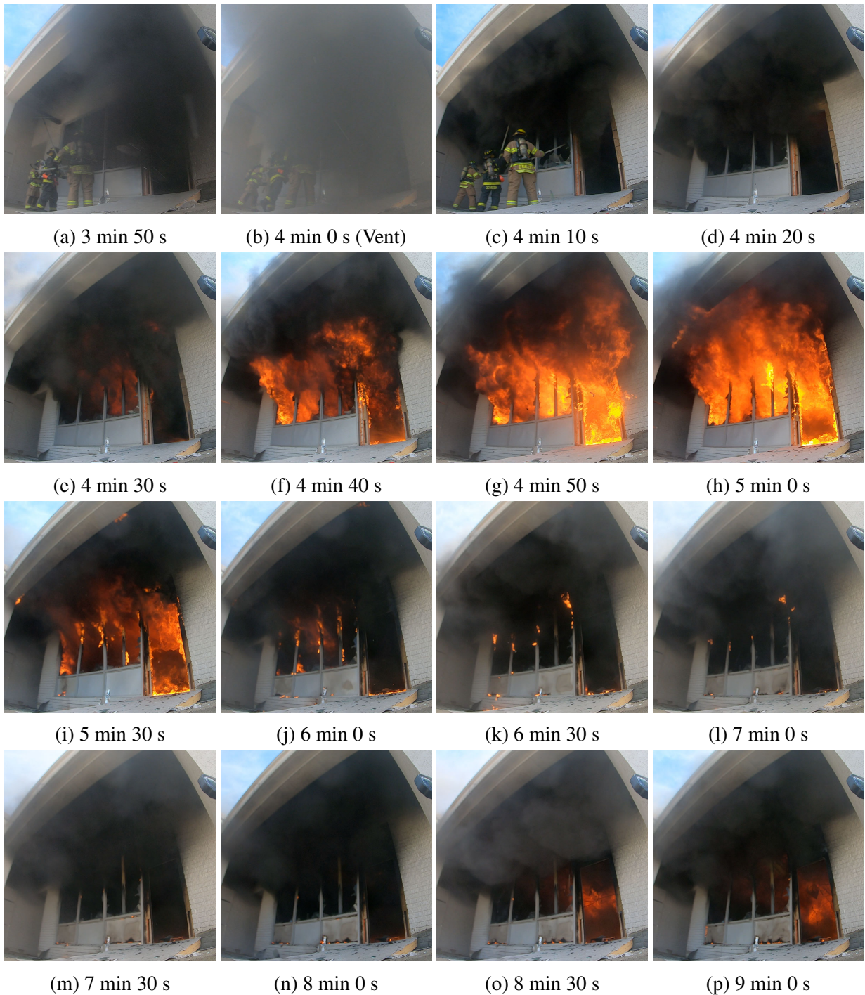
Figure 3.27: Changes in visible fire from side A after horizontal ventilation of glass in Experiment 3. Rows 1 & 2 show rapid changes from 10 s before ventilation to 1 min after (3 min 50 s to 5 min). Rows 3 & 4 show the transition into a temporary decay phase and subsequent regrowth over the following 4 min.
