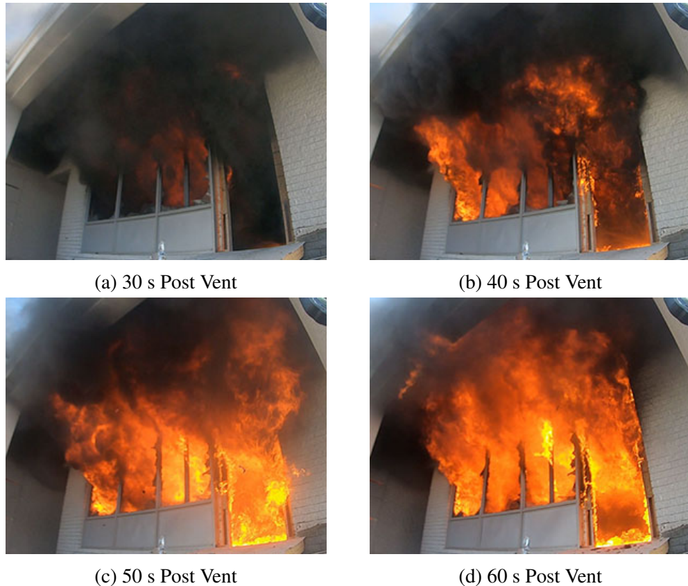
Figure 4.6: Sequential images showing the front of the unit starting 30 s after the ventilation of the front windows in Experiment 3. Images continue until 60 s after window ventilation had occurred.
