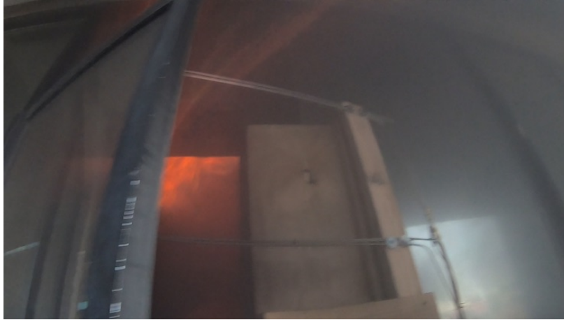
Figure 3.7: Flames exhausting from the front door captured by the helmet camera of the firefighter who closed the door during Experiment 1.
