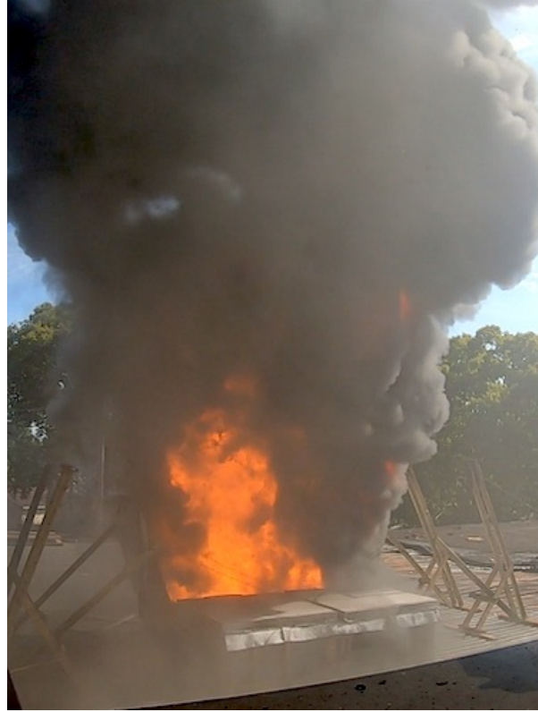
Figure 3.73: Image of the open BC and CD roof vents 30 s after ventilation occurred (6 min after ignition) during Experiment 7. The image was taken from the AB corner looking toward the CD corner.
