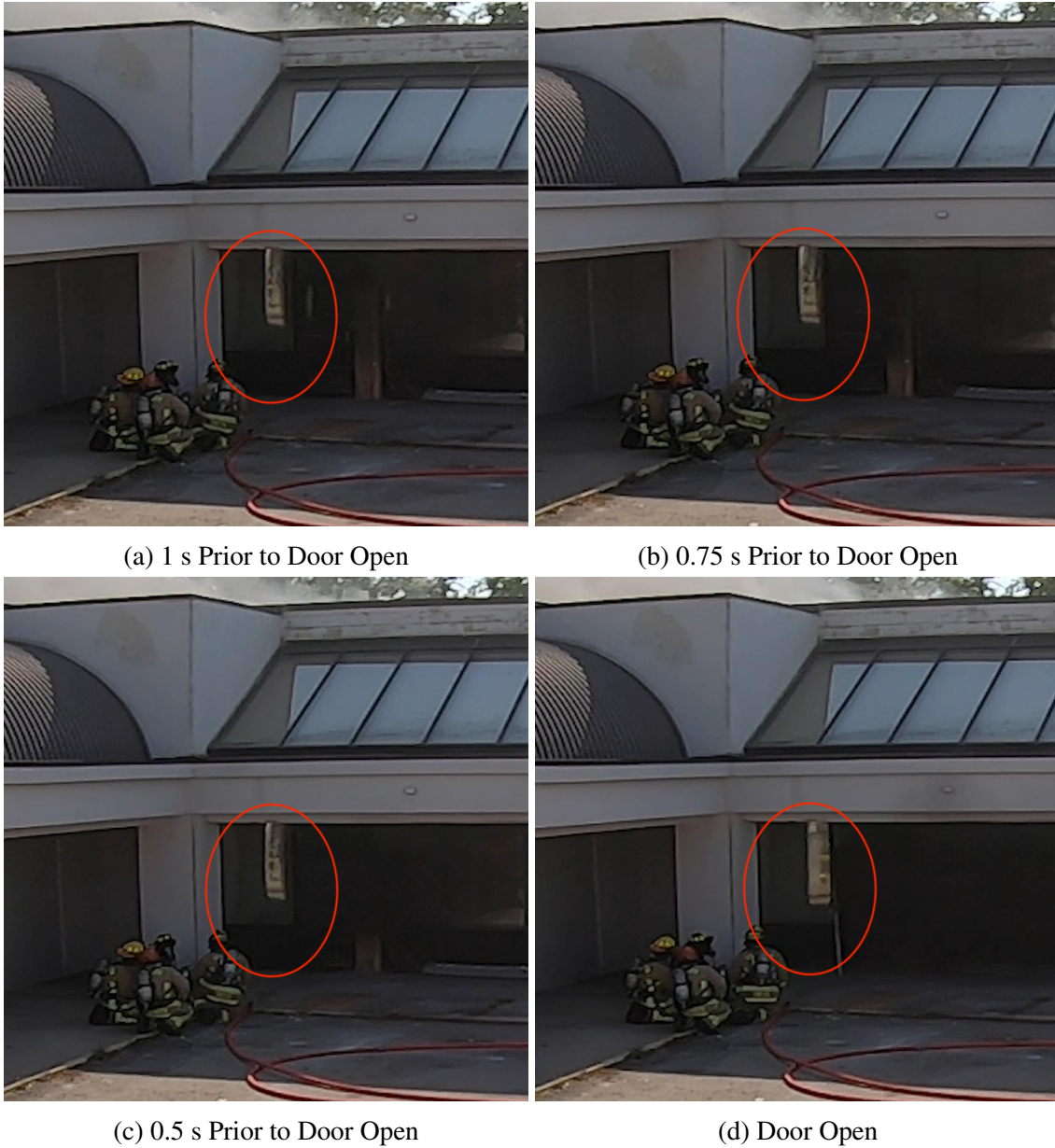
Figure 4.28: A series of images that show the pressure rise in Experiment 1 from 1 s prior to the door opening to the door opening. The reflection in three images prior to the door open show an outward bow of the glass, an indication of built-up pressure in the unit. Following the door opening, the reflection flattened out as the pressure inside the unit dropped.
