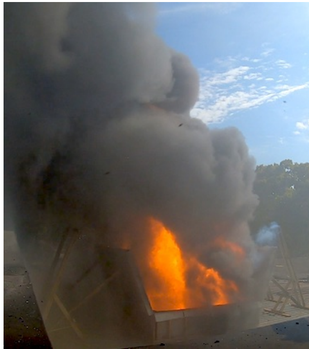
Figure 3.74: An image of the roof vents 10 s after ventilation occurred ( 7 min 40 s after ignition) during Experiment 7. Image was taken from the AB corner looking toward the CD corner.
