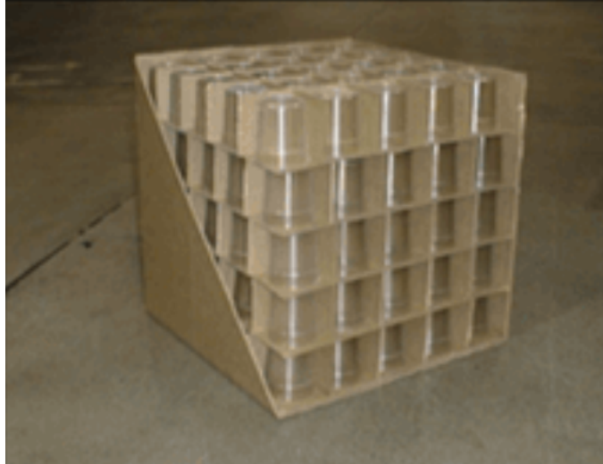
Figure 2.20: Image of the internal configuration of the plastics cups and cardboard in side a Group A plastic commodity box. The exterior cardboard has been cut away to reveal the internal structure.
