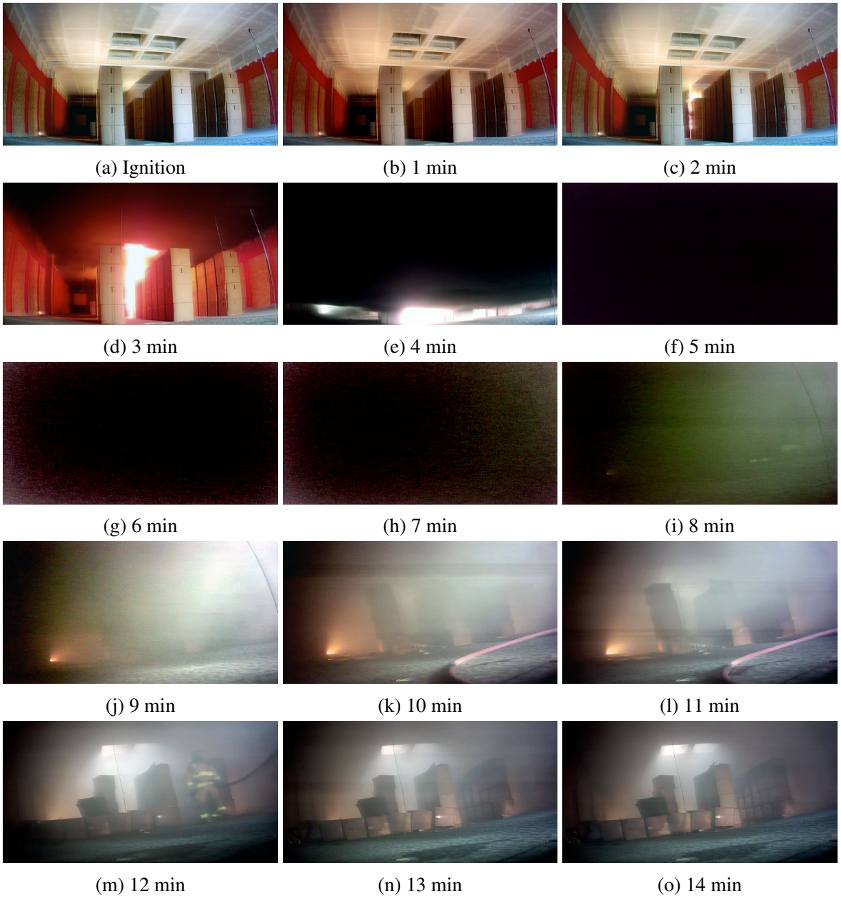
Figure 3.45: Sequential interior images during Experiment 5 looking toward side C from side A.
