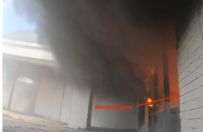
Figure 3.18: Image and approximate location of the neutral plane in the openings on the front of Unit 1078 during Experiment 2 following the ventilation of the AD left and center window panes 18 min after ignition. The red line approximates the height of the neutral plane.
