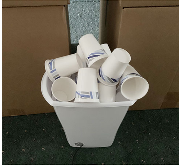
Figure 2.21: Image of the ignition source utilized in these experiments. The source consisted of wax paper cups and newspaper in a plastic trash can.
