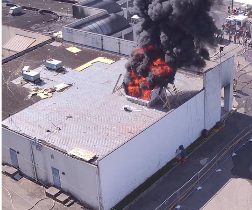
Figure 3.62: A drone image of the roof vents, looking from the BC corner toward the AD corner 10 s prior to suppression (9 min 14 s after ignition) in Experiment 6.
