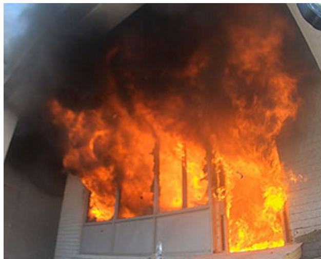
Figure 5.3: An image from Experiment 3 after all of the front windows were opened during the initial growth of the fire.
