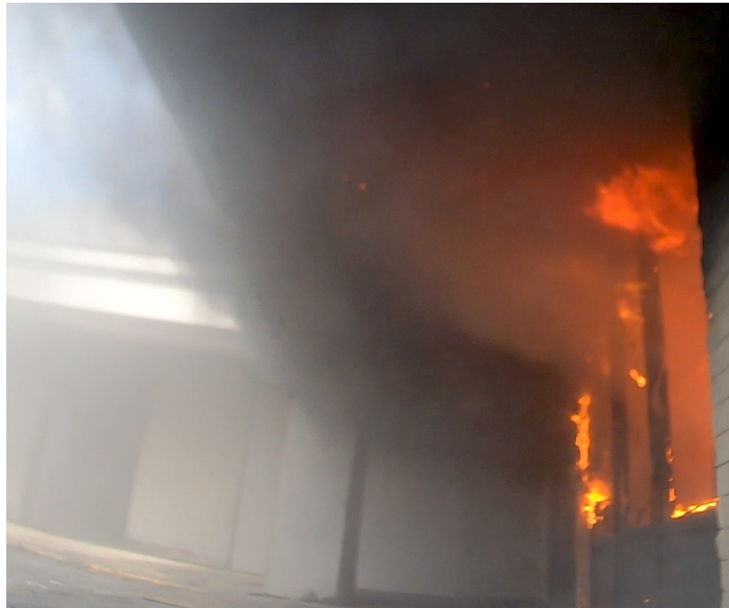
Figure 4.4: An image of flames venting out of the open front windows and door 18 min after ignition (Experiment 2).
