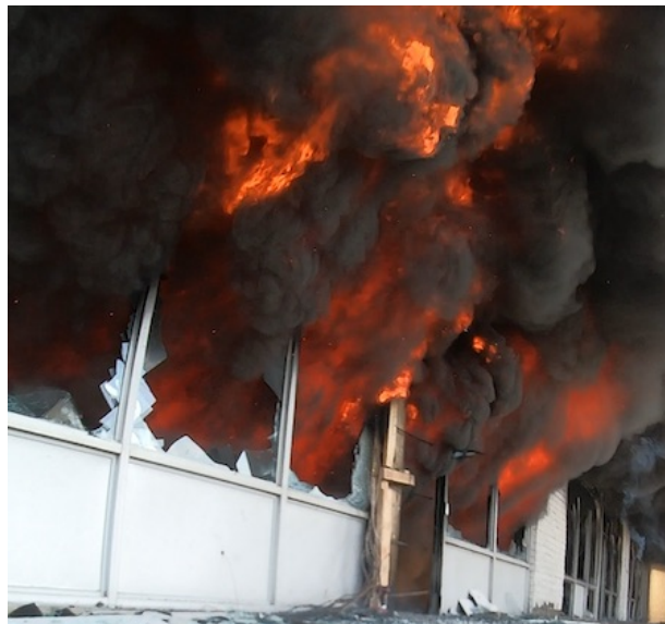
Figure 4.16: An image of flames venting out of the open front windows and door 1 min after horizontal ventilation, 5 min after ignition (Experiment 7).
