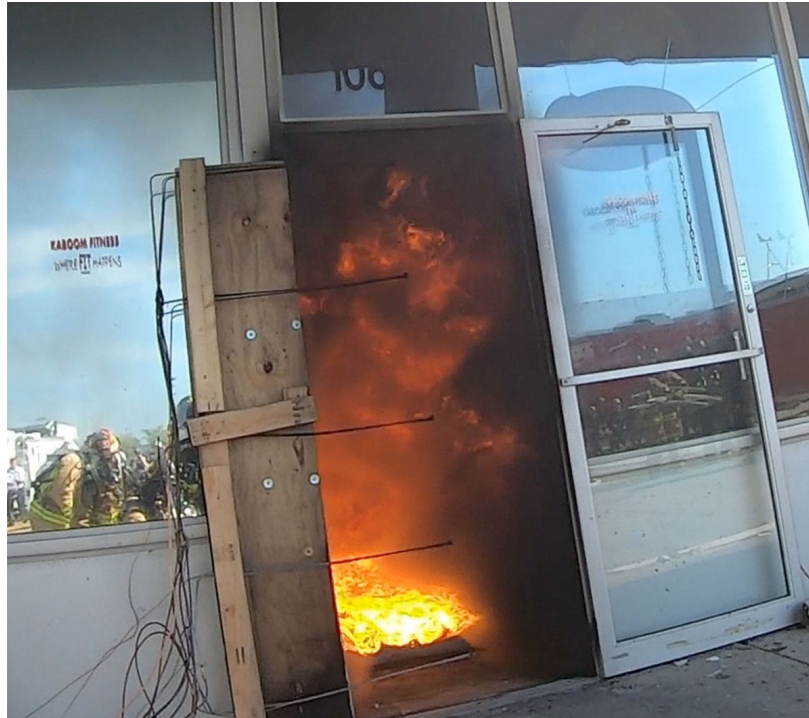
Figure 3.61: Flames at the front door 14 s prior to suppression (9 min 10 s after ignition) in Experiment 6.
