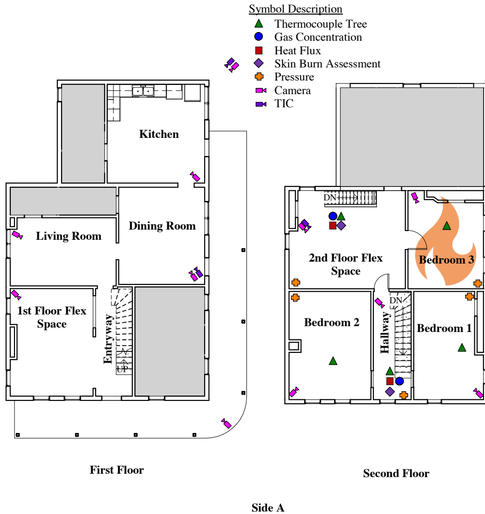
Figure 3.101: Instrumentation and floor plan for Experiment 9. The gray areas were isolated from the remainder of the structure and utilized as space for instrumentation.
