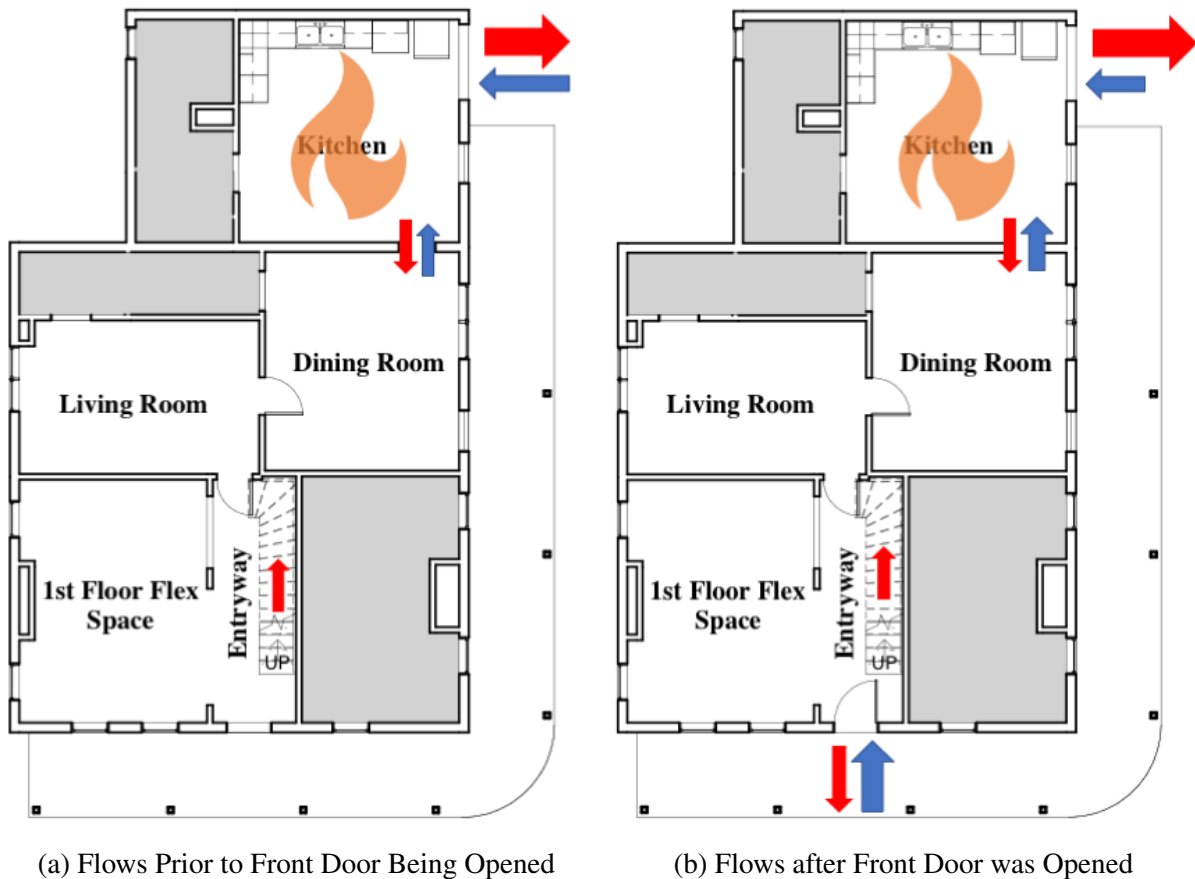
Figure 3.227: Changes in flow path for Experiment 18. Red arrows indicate flow out of the compartment, blue arrows indicate entrainment into the compartment, and the sizes of the arrows indicate the relative magnitude of the flow through each opening.
