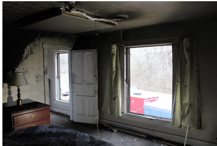
Figure 3.30: Interior vertical ventilation opening for Experiment 3.
