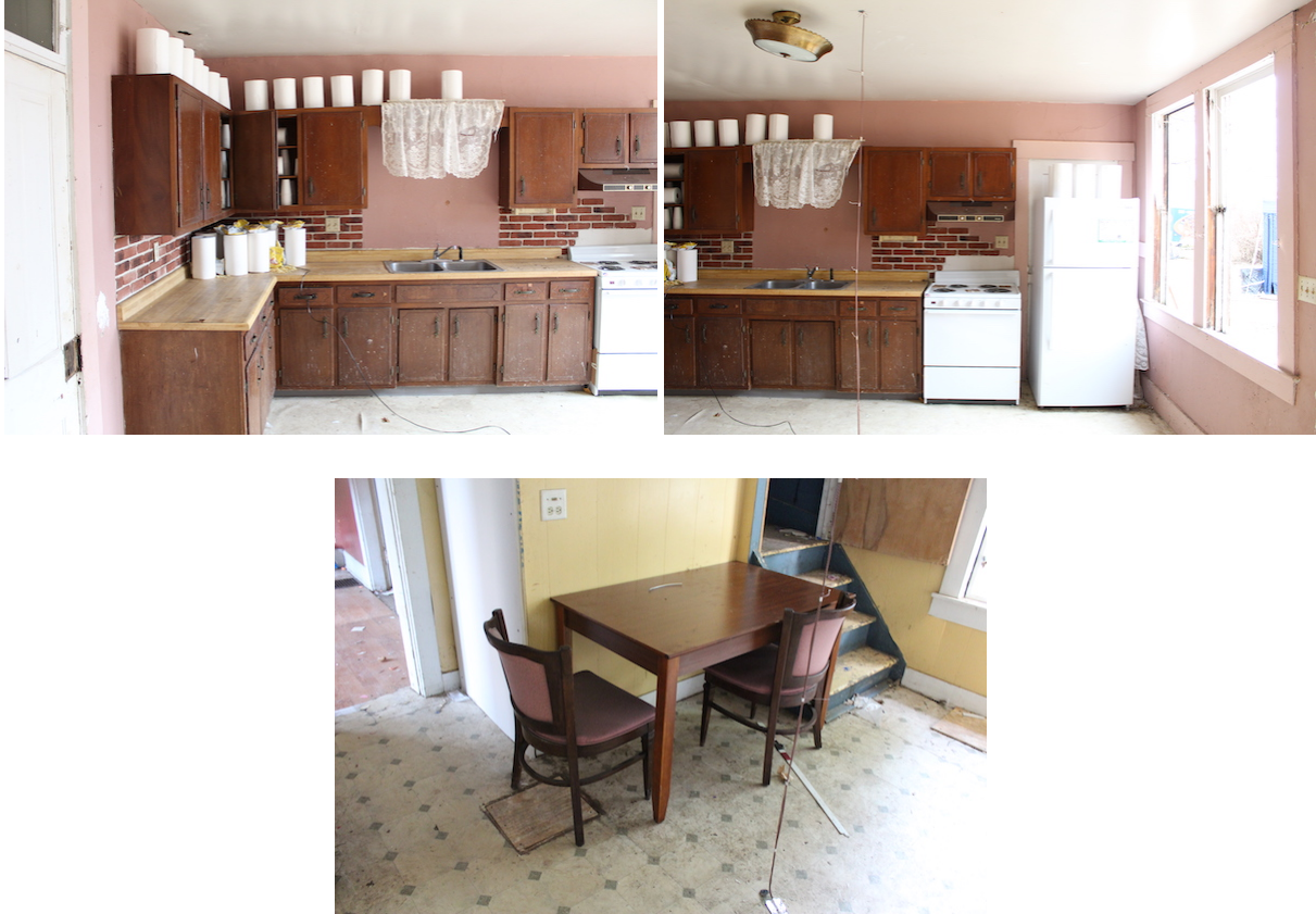
Figure 2.2: Representative kitchen fuel package containing cabinetry, a refrigerator, a range, a dining room table, two chairs, and ignition fuel package of a coffee maker, bags of potato chips, and paper towel rolls.
