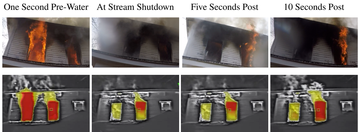
Figure 4.21: Visual representation of the effect of the initial water application on the fire room where the ceiling has failed for Experiment 14. Standard video from firefighters helmet from the A side(top), and infrared video from the A side (bottom). The columns are 1 s prior to water application (left) at the point the stream was shut down (left middle), 5 s post water application (Right Middle), and 10 s post water application (right).
