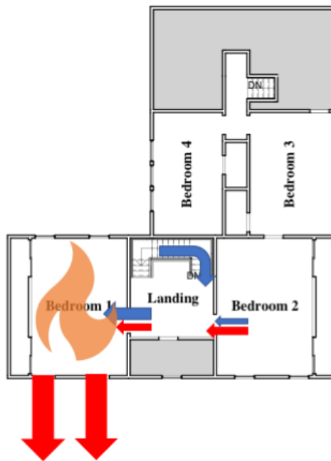
(c) During Hydraulic Ventilation
