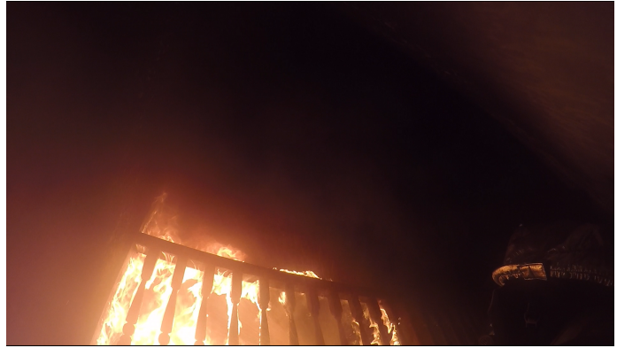
Figure 5.5: Initial suppression from stairway. From a position on the stairway (shown in isometric view, left), the nozzle firefighter applied water through the banister (right), dropping fire room temperatures.
