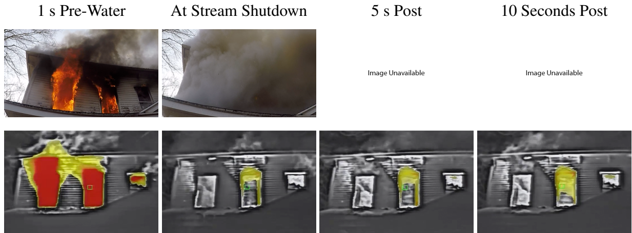
Figure 4.23: Visual representation of the effect of water application using a lintel suppression for Experiment 14. Standard video from firefighters helmet (Top), and infrared video from A/B corner (Bottom). The columns are 1 s prior to water application (left) at the point the stream was shut down (left middle), 5 s post water application (right middle), and 10 s post water application (right).
