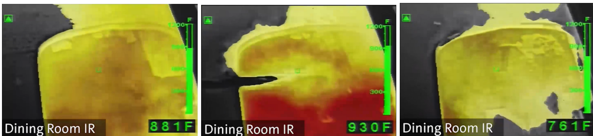
Figure 5.8: Thermal imaging views of ineffective water application in Experiment 16. Camera is in the dining room, directed toward the kitchen. Images show start of flow into dining room wall (left), start of flow into fire room (middle), and 40 s after start of water flow (right).
