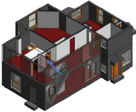
Figure 5.5: Initial suppression from stairway. From a position on the stairway (shown in isometric view, left), the nozzle firefighter applied water through the banister (right), dropping fire room temperatures.
