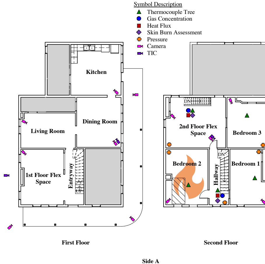
Figure 3.162: Instrumentation and floor plan for Experiment 14. The gray areas were isolated from the remainder of the structure and utilized as space for instrumentation. The diagonal hatched box indicates the size and location of the failed ceiling.
