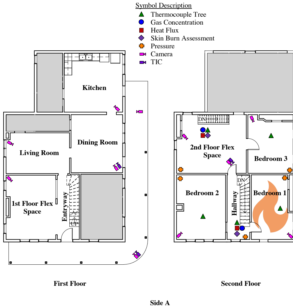
Figure 3.62: Instrumentation and floor plan for Experiment 6. The gray areas were isolated from the remainder of the structure and utilized as space for instrumentation.
