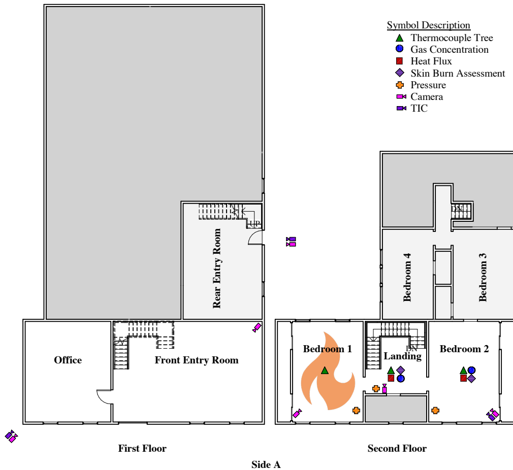
Figure 3.16: Instrumentation and floor plan for Experiment 2. The dark gray areas were isolated from the remainder of the structure and utilized as space for instrumentation. The light gray areas indicate the sub-structure not utilized for this experiment.
