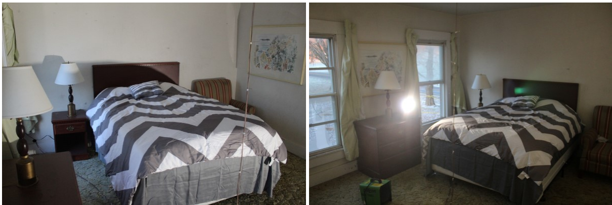
Figure 2.1: Representative bedroom fuel package containing bed frame, headboard, box spring, mattress, and associated bedding as well as a nightstand, dresser, sofa chair, lamp and shade, and pictures.
