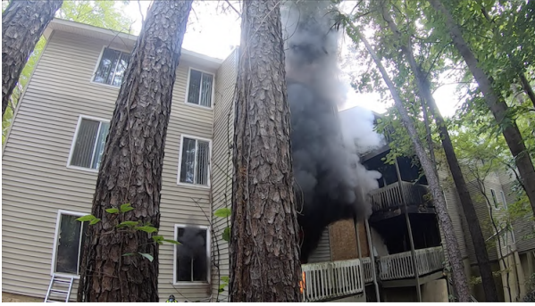
(a) 461 s Post Ignition – Kitchen Window Vented
