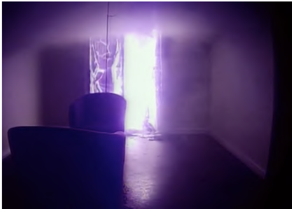
(c) 653 s Post Ignition – Left Pane Failure
