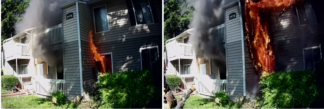
(a) Kitchen Window Failing (709 s)
