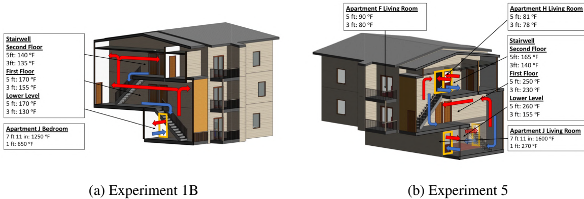
Figure 4.20: Fire apartment and stairwell temperatures for Experiments 1B and 5. Experiment 5 includes target apartment (F and H) living room temperatures. Data are presented 340 s post-ignition, which was prior to Apartment H door closing in Experiment 5. Red arrows indicate the flow of combustion products, blue arrows indicate the flow of fresh air, and the size of the arrows indicate the relative magnitude of the flow. Yellow boxes indicate ventilation openings.
