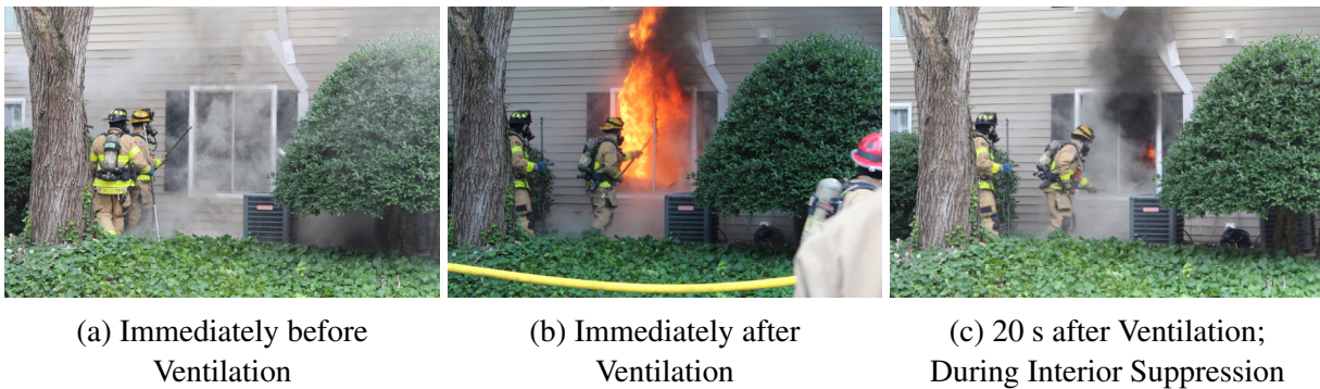
Figure 3.27: Images of the fire room (bedroom) window in Experiment 1C being broken to provide horizontal ventilation in coordination with interior suppression.
