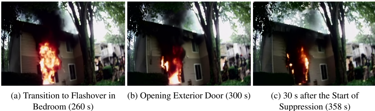
Figure 3.65: Images of the fire room (bedroom) window in Experiment 2A at flashover and during firefighter operations.
