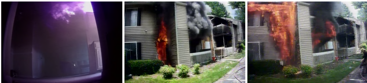
(a) Interior Conditions at Time of Second Ignition (420 s) (b) Exterior Conditions at Time of Kitchen Flashover (632 s) (c) Exterior Conditions at Time of Living Room Flashover (711 s)
