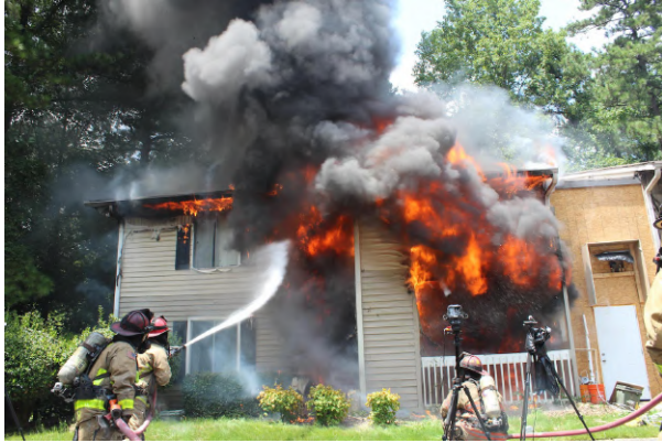
(a) Start of Water Application to Eaves Above Kitchen Window (768 s)
