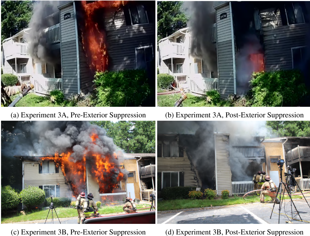
Figure 5.28: Fire conditions on exterior of structure immediately before and immediately after exterior fire control in Experiments 3A and 3B. The exterior suppression action utilized approximately 94 gal and 25 gal in Experiments 3A and 3B, respectively.
