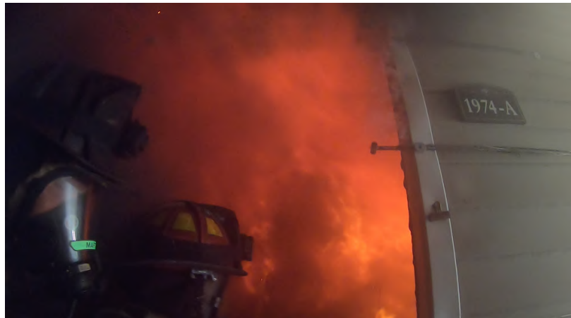
Figure 5.22: Conditions in the fire apartment at the time of door open for Experiment 3A.
