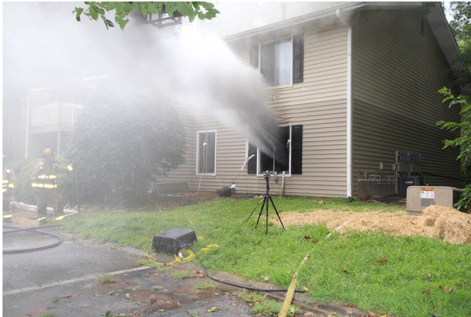
Figure 3.39: Image of hydraulic ventilation from the bedroom (fire room) window in Experiment 1D.
