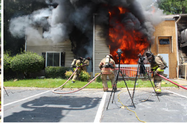
(b) During Water Application through Kitchen Window (Started at 777 s)
