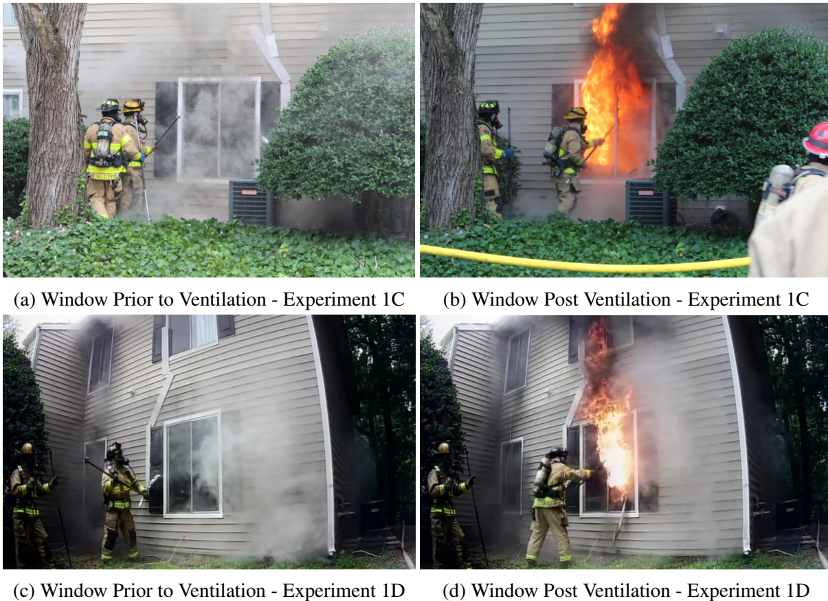
Figure 4.10: Changes in exterior conditions before and after horizontal ventilation in Experiments 1C and 1D.
