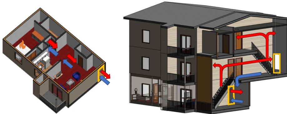
(b) After Opening the Breezeway and Fire Apartment Door
