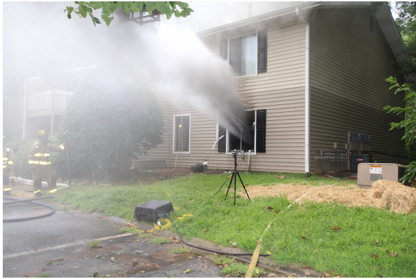
(a) Experiment 1D – Hydraulic Ventilation
