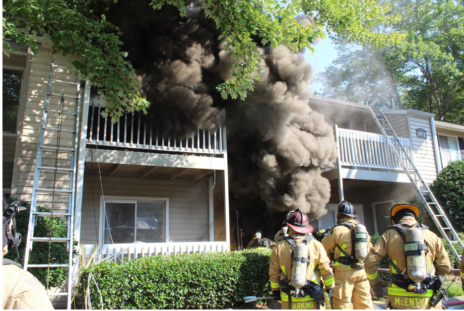
Figure 5.10: Conditions faced by the suppression crew as they opened the exterior breezeway door for entry and suppression in Experiment 5.
