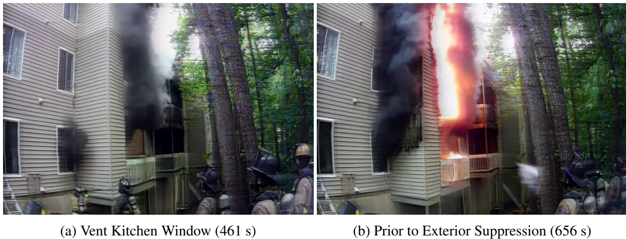
Figure 3.170: Images of the conditions on the side C exterior during firefighter interventions in Experiment 6.
